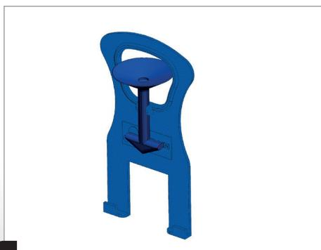
12 Siphon lifter with an attachment for the suction cup.
